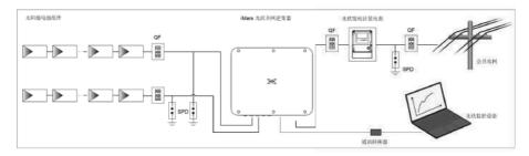
Fig 5.1 Schematic diagram of PV grid-connected system connection
