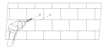
**Step 3:** Fix the hanging board. Clean the holes, use a rubber hammer to drive the expansion bolt into the hole, use a wrench to tighten the nut to fix the end of the bolt, then remove the nut, spring washer and flat washer, and then fix the wall mount plate to the wall and lock it with a tightening torque of 13N\*m<sub>o</sub>.
