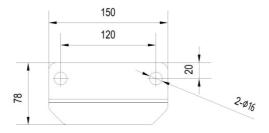
Fig 4.7 Dimensions of the mounting plate
