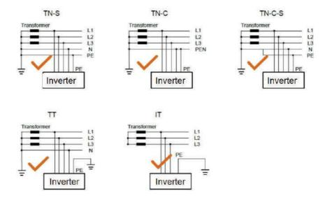
Fig 2.2 Grid forms supported by PV grid-tied inverters
