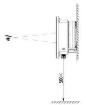
Fig4.3 Optimum installation height area
