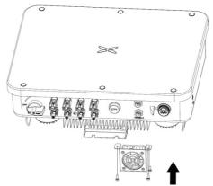
**Step 3:** Use a soft brush or vacuum cleaner to clean the fan. If the fan is damaged, follow step 4. **Step 4:** If the fan is damaged, remove the damaged fan and install the good fan to its original position.
