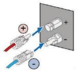
Fig 5.5 PV DC string connected to the inverter
