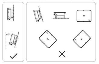
Fig 4.6 Installation position of inverter
