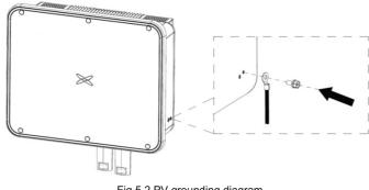
Fig 5.2 PV grounding diagram
