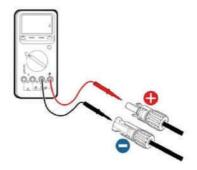
Fig 5.4 Measuring DC input voltage
