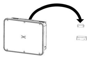
**Step 4:** Use an M4×12 screw to fix the inverter with the hole on the left side of the chassis and the wall mount, and the tightening torque is 2.5N\*m
