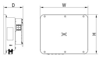
Figure 2.5 Outline dimensions of the inverter
