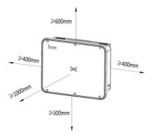
Fig 4.4 Installation spacing of inverter
