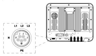
Fig 5.9 Three-phase inverter grid connection
