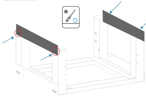
**Step 6**: Remove the guide rail, mount the side cover, fix the side cover to the connecting strip with M4 screws from the inner side.
