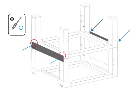
**Step 2**: Mount the connecting strip, fix the connecting strip (waist hole) to the bottom of the rack with M6 screws.
