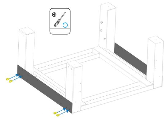
**Step 5**: Mount the racks in order to the required number of layers (up to three layers) according to the above method, ensure that the racks are aligned in all directions, then tighten the M6 screws (recommended torque 6N.m) on the rack connecting strip with a spanner.
