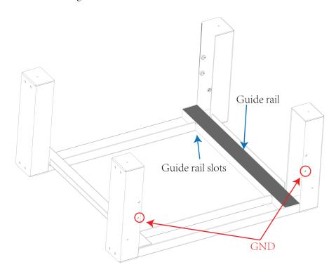
**Step 4**: Place the second layer rack, limit the positions with the guide rail slots, and fix the connecting strip (waist hole) to the bottom of the second layer rack. Note: The two adjacent layers of racks should be vertical aligned.
