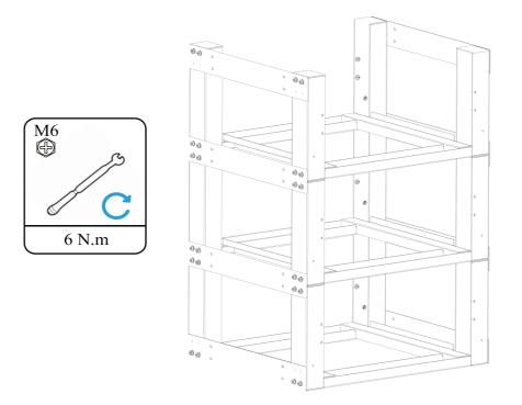
**Step 3**: Mount the connecting strip, fix the connecting strip (round hole) to the top of the rack with M6 screws.
